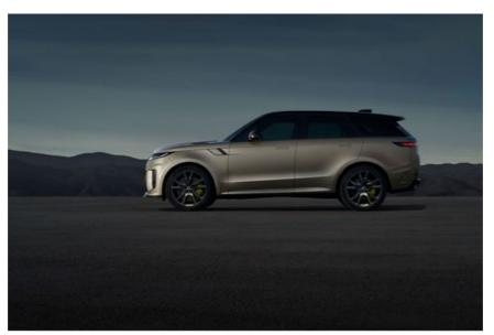
Carbon Revolution's ultra-lightweight 23-inch carbon fiber wheels on the Range Rover Sport SV weigh an average of 41% less than conventional 23-inch cast-alloy wheels, resulting in improvements to outright performance, handling and ride quality.
